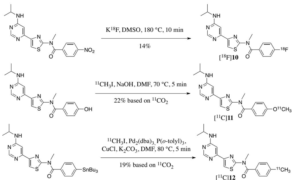
Fig. (6). Radiosynthesis of  $[^{18}\text{F}]\mathbf{10}$ ,  $[^{11}\text{C}]\mathbf{11}$  and  $[^{11}\text{C}]\mathbf{12}$ .
